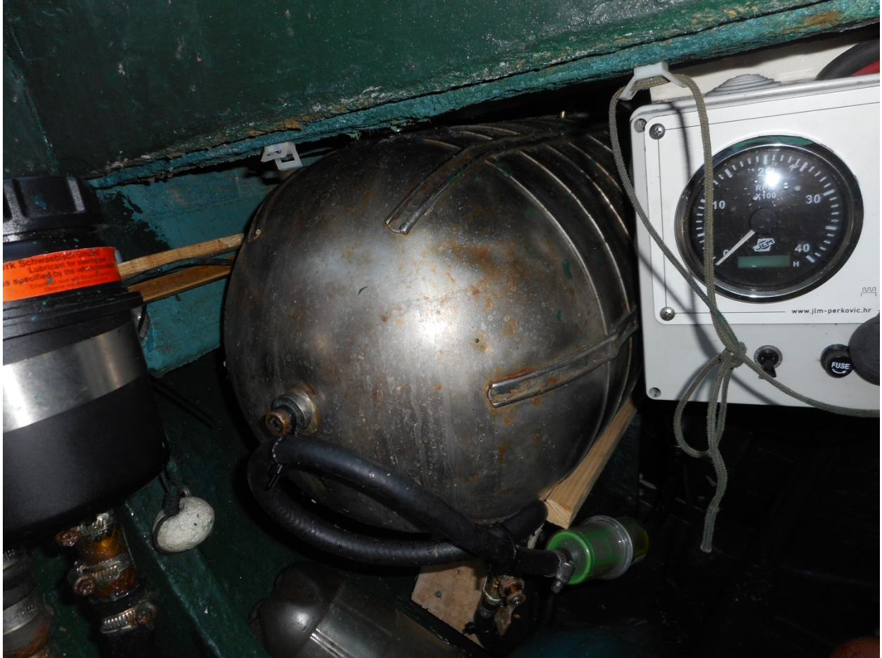
Oxygen tank from the B24J 4278519 that is used as fuel tank on old boat in Molunat
