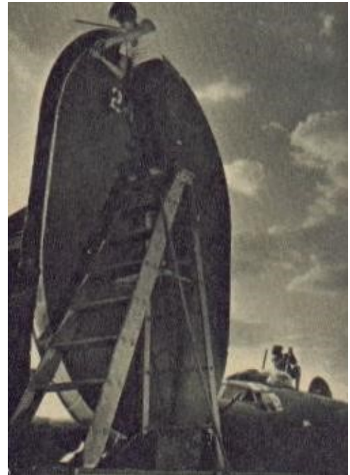
A de-icer boot comes off one of the twin rudders of a Liberator. Operational needs find the cow pasture mechanics skilled and ready upon notice.
