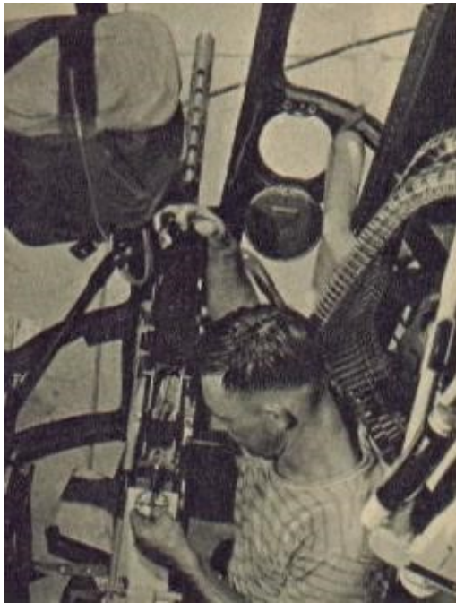
With a .50 caliber nose gun in place, a workman installs the sight – puts the loading rack in properly – checks the machine gun for proper movement.
