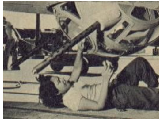
Fully retractable turrets being installed in the belly of a bomber. At the last station of the line, the ball turret gets its final glass panel polish.
