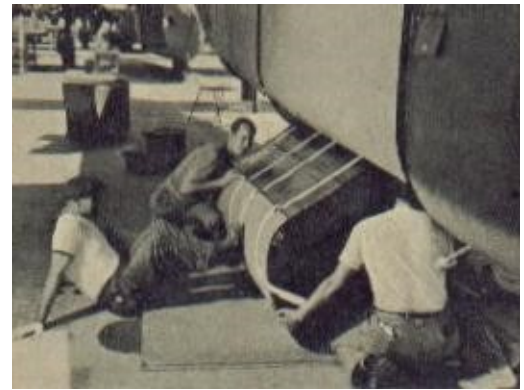
With the B-24's leaving for far flung fronts, extra bomb bay tanks are installed which can be dropped when the ship reaches its destination.
