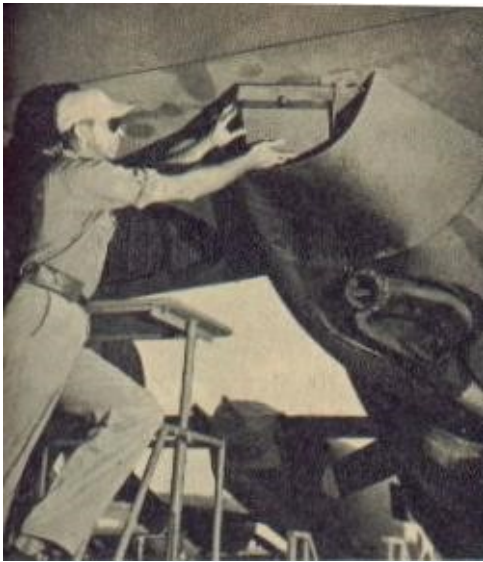
At the rear of a mighty Pratt and Whitney engine, a workman installs the "dust catcher" which will help lengthen the life of the engine in combat.
